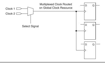
Adding multiplexing logic to the clock signal can create the problems addressed in the previous sections, but requirements for multiplexed clocks vary widely depending on the application. Clock multiplexing is acceptable when the clock signal uses global clock routing resources, if the following criteria are met:
