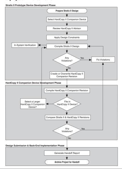
Prototype your HardCopy II design by selecting and then compiling a Stratix II device in the Quartus II software.
