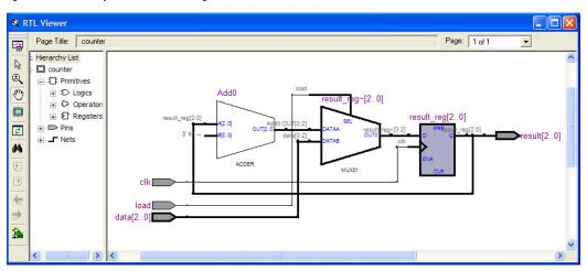
Figure 12–3. Example Schematic Diagram in the RTL Viewer
