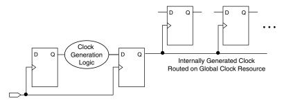
Registering the output of combinational logic ensures that the glitches generated by the combinational logic are blocked at the data input of the register.
