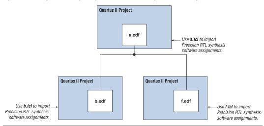
Figure 10–4. Design Flow: Using Multiple EDIF Files with Multiple Quartus II Projects
