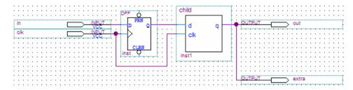
In this case, the software does not perform output register packing. If there is a Fast Output Register assignment on pin out, the software issues a warning that the Fitter can't pack the node to an I/O pin because the node and the I/O cell are connected across a design partition boundary.
