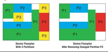
Performing this placement is very difficult. The Fitter may not be able to find any legal placement for the logic in partition **P3**, even if it was able to do so in the initial compilation. If the Fitter does find a legal placement, the results are probably sub-optimal.
