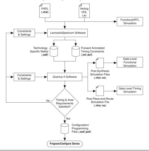
Figure 9-1. Recommended Design Flow Using LeonardoSpectrum and Quartus II Software
