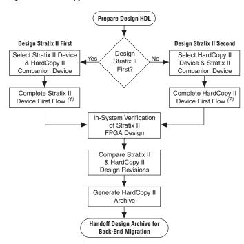
Figure 4-1. HardCopy II Flow in Quartus II Software
