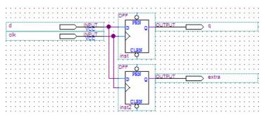
Figure 2-20. Modified Top-Level Design from Figure 2-18 Connecting Two Output Ports to Output Pins
