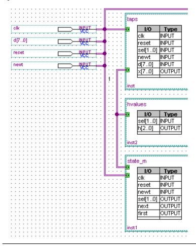
Figure 3-12. Blocks and Pins Connected with Conduits
