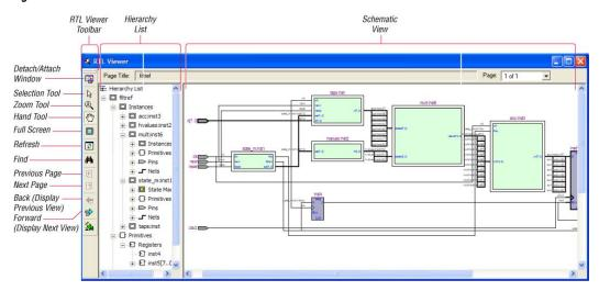
Figure 12-2. RTL Viewer Window and RTL Toolbar
