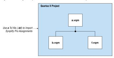
Figure 7-4. Design Flow Using Multiple VQM Files with One Quartus II Project
