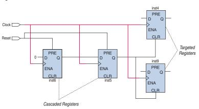
Figure 5-10. Active-Low Reset Ports
