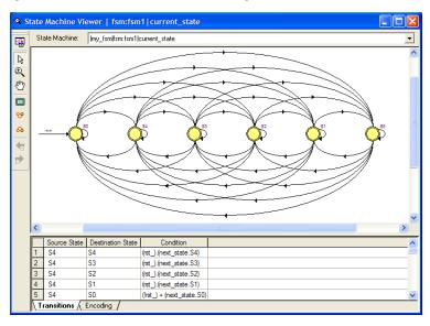
2. You can analyze this state machine instance using the state machine diagram, transition table, and encoding table. Clearly something is wrong with the state machine because every state has a transition to every other state. After inspecting the state machine behavior, you determine that in this scenario, the designer forgot to create default assignments for the next state (that is, next\_state = current\_state if the conditions are not met).
