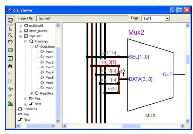
Figure 12–28. Rollover in the RTL Viewer and Technology Map Viewer
