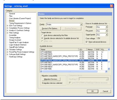
Figure 4–18. Selecting a HARDCOPY\_FPGA\_PROTOTYPE Device
