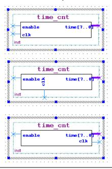
Figure 3–11. Various Port Position for a Symbol
