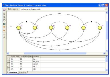
Figure 12–34. State Machine Viewer Showing Correct Transitions
