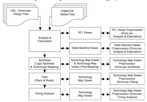
Figure 12-1. Quartus II Design Flow Including the RTL Viewer and Technology Map Viewer
