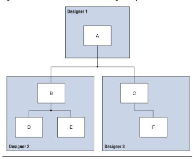
Figure 9-3. Block-Based and Team-Based Design Example
