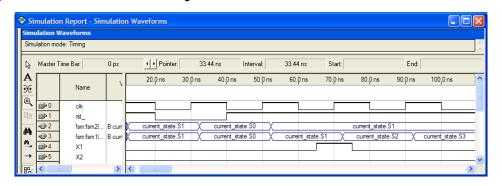
Figure 12-35. Simulation Result Showing Correct States
