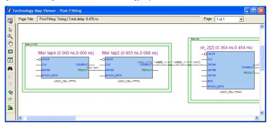
Figure 12–25. Timing Path Schematic in the Technology Map Viewer
