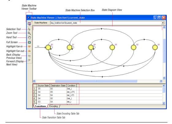
Figure 12-5. State Machine in the State Machine Viewer
