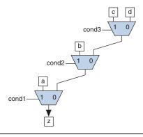
An *N*-input priority multiplexer uses a LUT for every 2:1 multiplexer in the chain, requiring *N*-1 LUTs. This chain of multiplexers generally increases delay because the critical path through the logic traverses every multiplexer in the chain.
