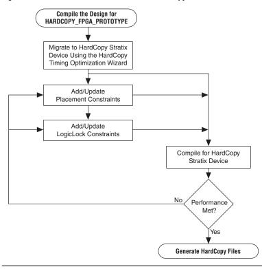
Figure 4-22. Placement Constraints Flow for HardCopy Stratix Devices
