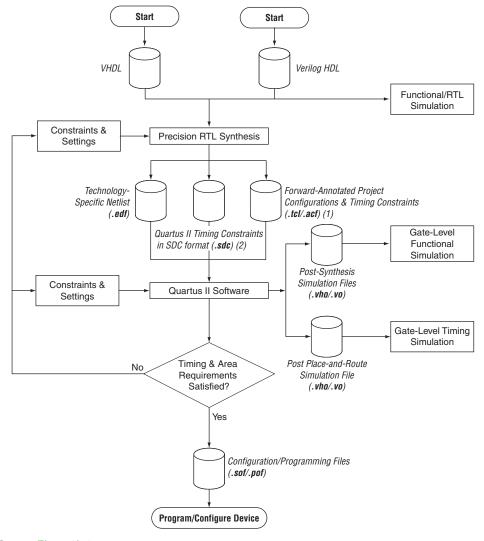
Figure 10–1. Design Flow Using the Precision RTL Synthesis Software and Quartus II Software
