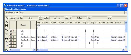
Figure 12–30. Simulation Result Showing Undefined States
