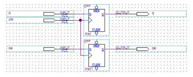
Figure 2–24. Top-level Design Instantiating the Subdesign in Figure 2–25 to Drive Output Enable Logic
