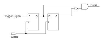
Figure 5-3. Recommended Pulse-Generation Technique
