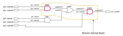
Figure 12–19. Between Selected Nodes Filtering Between inst2 and inst3
