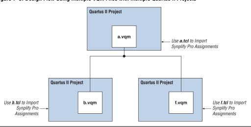
Figure 7-5. Design Flow Using Multiple VQM Files with Multiple Quartus II Projects
