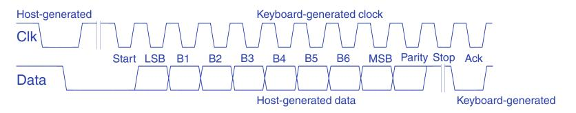
Host brings Clock low, then Data low to indicate transfer to keyboard, then releases Clock (rises).
