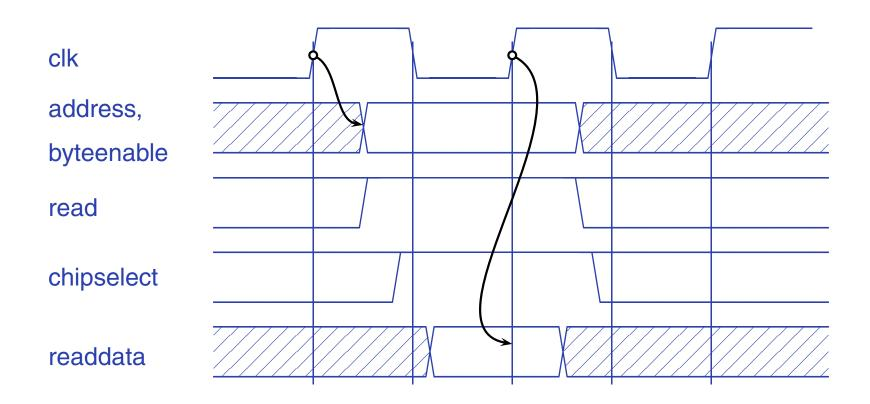
Bus cycle starts on rising clock edge. Data latched at next rising edge. Such a peripheral must be purely combinational.
