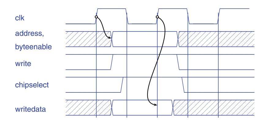
Bus cycle starts on rising clock edge. Data available by next rising edge. Peripheral may be synchronous, but must be fast.
