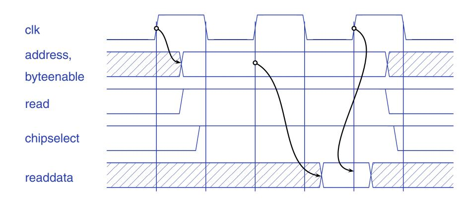
Bus cycle starts on rising clock edge. Data latched two cycles later. Approach used for synchronous peripherals.
