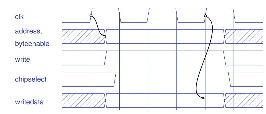
Bus cycle starts on rising clock edge. Peripheral latches data two cycles later. For slower peripherals.
