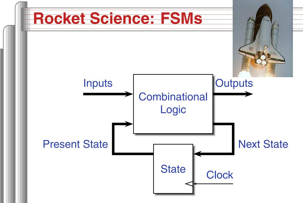
This is a *Mealy* FSM: outputs may depend directly on inputs.
