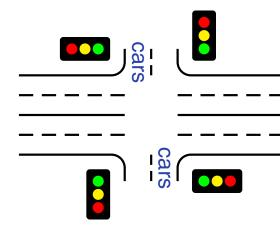
This controls a traffic light at the intersection of a busy highway and a farm road. Normally, the highway light is green but if a sensor detects a car on the farm
