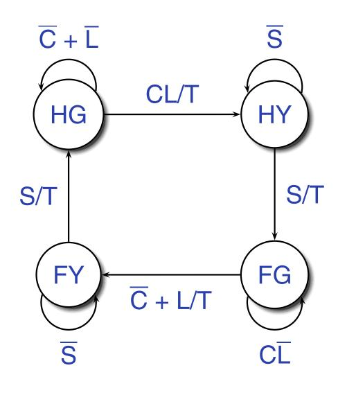
C: Car sensor S: Short timeout L: Long timeout T: Start timer Hwy St **Farm** HG G R HY R Y FG R G FY R
