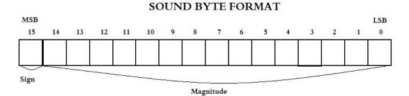
The most significant bit of the sound byte is the sign bit. If this bit is 0 (positive number), then the resulting integer sent to the software ranges from 0 to 32,767 in order of increasing magnitude. If it is 1 (negative), then the integer ranges from 32,768 to 65,535 in decreasing magnitude, as a two's complement system is used. This relation of the physical bits in the sound byte to the integer passed to the software will be important for the frequency algorithm implemented in the software.
