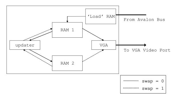
The vga\_raster in essence serves three functions. The first is to accept the initial conditions from the Nios Processor across the Avalon bus. The second is to take the current state of the board and output it to the screen through the 'VGA' block. The last, but equally important job of the vga\_raster is to update the current state of the board and output the next generation to another block of RAM.
