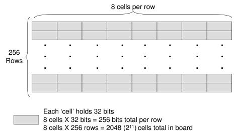
Each of our cells in RAM holds 32 bits. Since our board is 256 bits in length and width, we can think of this as having 8 cells of 32 bits per row and 256 rows in total.
