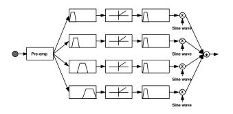
Figure 1: *Example of 4-channel speech processing for the CI simulation.*
