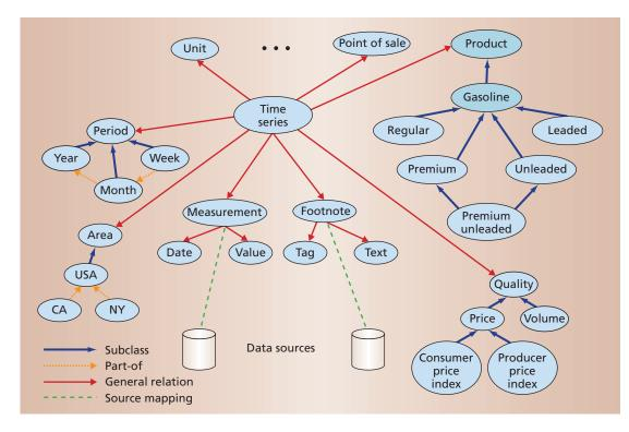
Figure 2. Fragment of an EDC domain model describing timeseries data about different gasoline products. Each concept models a class of database contents. The user frames queries in terms of these concepts and their variants.
