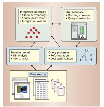
Figure 1. The EDC system architecture includes an integrated ontology, a user interface, a query processor, a domain model, and the data sources.
