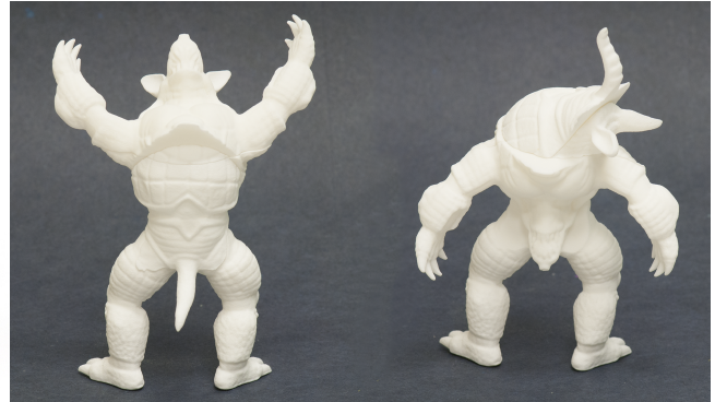
Figure 1: Twisty Armadillo. (left) A twisty puzzle in the shape of an ARMADILLO whose rotation axes are placed along a triangular prism. (right) The output of our algorithm was fabricated, assembled, and scrambled into contorted poses. The different parts of the model, such as the arms and legs, were deformed so that they do not collide with one other regardless of the configuration of the puzzle.
