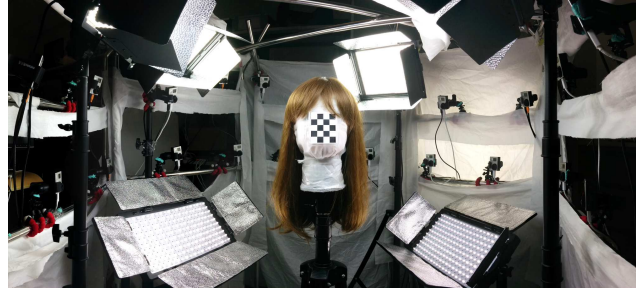
Figure 2: Our dynamic hair acquisition setup consists of 21 GoPro cameras and six LED arrays.
