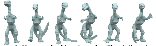
Figure 3: Unconstrained inertia modes. First six linear inertia modes of an unconstrained model (see the supplemental video).
