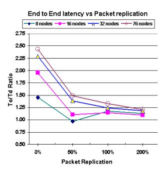
Figure 6: End-to-end average latency results for the index page and a collection of pages for www.cnn.com. The different points denote the change in the end-to-end latency through the overlay  $(T_o)$  when compared to the direct connection  $(T_d)$ . Different lines represent different sized overlays. Increasing the replication factor, and for larger networks, we get lower average latency results because of the multipath effect on the transmitted packets.
