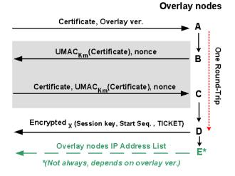
Figure 4: Key & Ticket Establishment protocol: The client sends node A his certificate. A immediately redirects the request to B, in the two-round-trip protocol, or to D for the one-round-trip protocol. The four-message protocol is more resilient against computational attacks since it ensures the client's liveness before generating an encrypted version of the ticket. A  $5^{th}$  message is transmitted when the client's version for the list overlay nodes is old.
