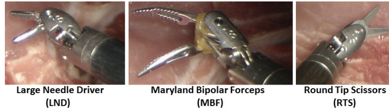
Fig. 7. Images of the three types of tool dealt with successfully in this paper. We train only on the LND (left), and are able to track on all three, including the MBF (middle) and RTS (right).
